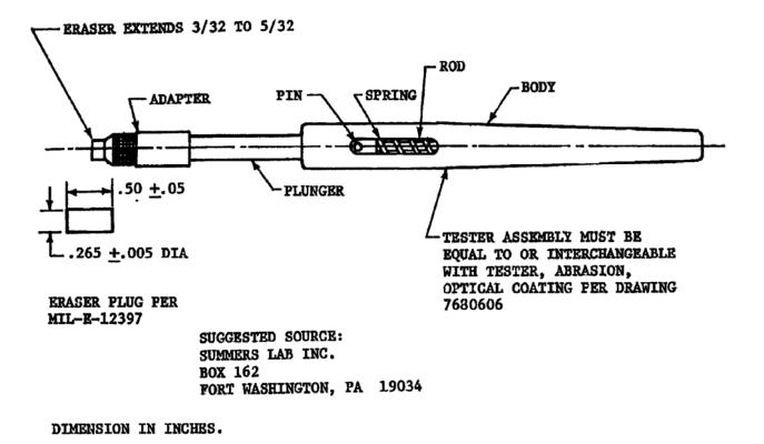
FIGURE 5. Eraser abrasion tester assembly and eraser plug.
