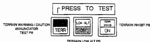
Fig. 3 Zoom of EGPWS annunciators and pb's (I-panel) - typical
